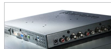
Ultimate video versatility, including passive looping BNC video for multiple display connections
